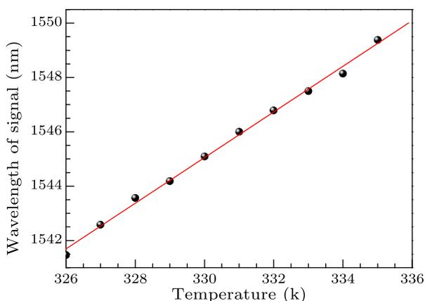
**Fig. 4.** Central wavelength of signal photons plotted versus the temperature of the PPLN crystal.
