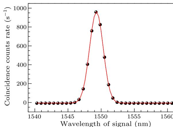
**Fig. 2.** Spectrum of signal photons.
