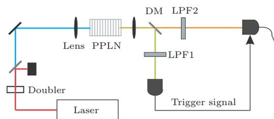
**Fig. 1.** The experimental setup of our source. Laser: Ti:sapphire laser, doubler: frequency doubler, PPLN: periodically-poled LiNbO<sub>3</sub>, DM: dichroic mirror, LPF1 and LPF2: low pass filter,  $L_p$  and  $L_s$ : lens, Si-APD: single-photon detector made of silicon avalanche photon detector, SPD: InGaAs-InP avalanche photodiodes operating in a gated Geiger mode.
