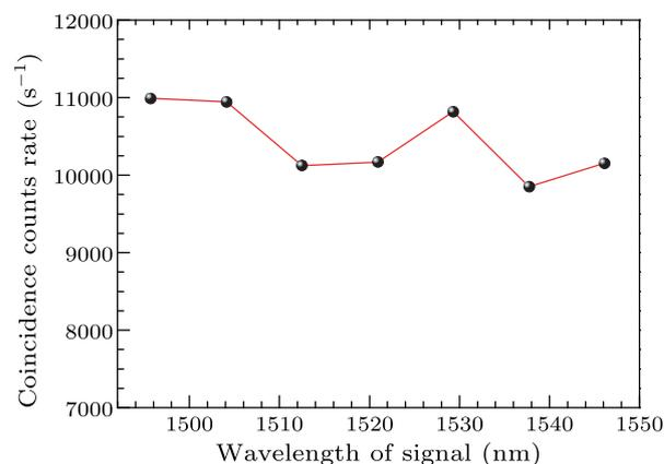
**Fig. 3.** Coincidence count rate versus the central wavelength of signal photons.
