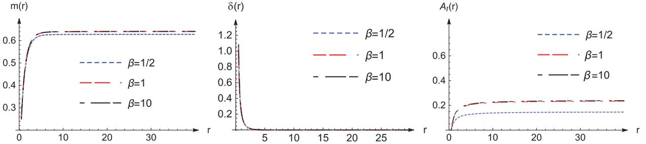
Fig. 2: Numerical solutions of Group II for  $m(r)$ ,  $\delta(r)$  and  $A_t(r)$  with  $Q = 0.16$  and  $r_0 = 0.5$ . The values of expansion coefficients  $(\delta_0, m_1)$  are  $(0.983, 0.399)$ ,  $(1.064, 0.410)$  and  $(1.086, 0.410)$  for  $\beta = 1/2, 1$  and  $10$ , respectively. Moreover, the mass function  $m(r_0)$  equals  $\frac{r_0}{2} = 0.25$ .
