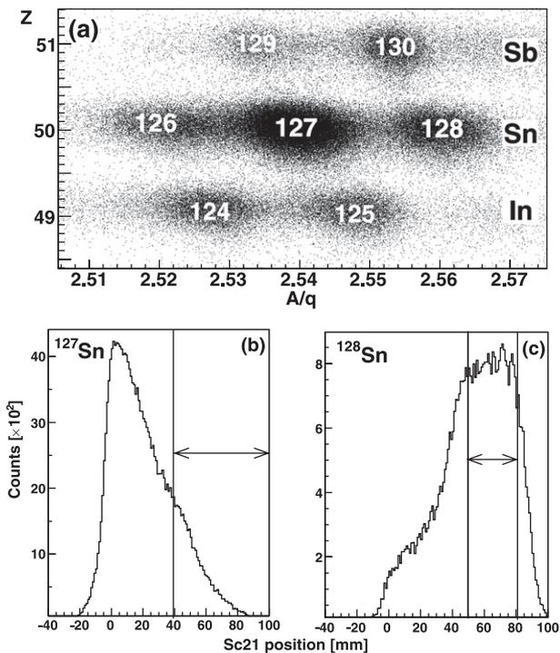
Fig. 2: (a) Ion identification plot. The spots corresponding to different isotopes are labelled with the isotope notation; (b) longitudinal momentum distribution for  $^{127}\text{Sn}$ ; (c) longitudinal momentum distribution for  $^{128}\text{Sn}$ . The momentum distribution is measured with Sc21. The vertical lines in (b) and (c) indicate the momentum selection, which was used in the data analysis.
