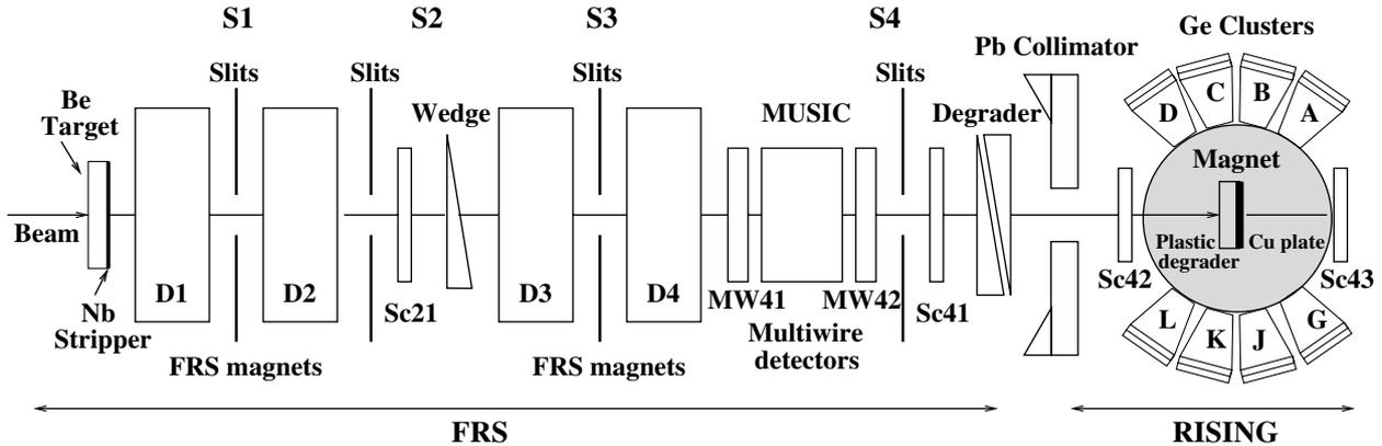
Fig. 1: Schematic view of the experimental set-up (see text): the fragment separator (FRS) with the beam-tracking detectors, the RISING  $\gamma$ -ray detectors (A–D) and (G–L), the electromagnet and the implantation detectors.
