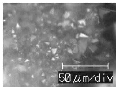
Fig. 5. Transparent GaN single crystals grown near the gas-liquid interface in Ca 5 mol% mixed flux.
