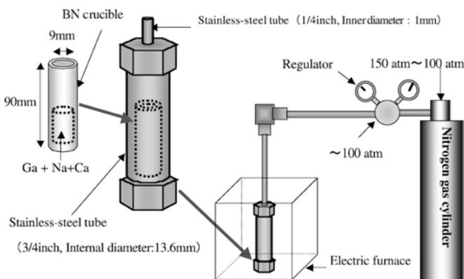
Fig. 1. Schematic illustration of experimental apparatus.
