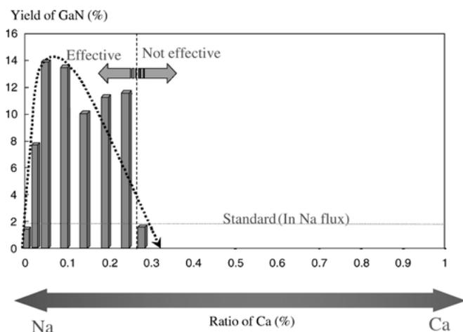
Fig. 2. Relationship between flux composition and yield of GaN grown in various compositional fluxes. Yield is indicated as ratio of GaN crystals grown in flux against metallic Ga of starting material.
