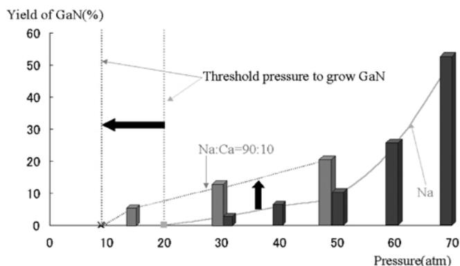
Fig. 3. Changes in yields of GaN synthesized in pure Na flux and Ca 10 mol% mixed flux according to the reaction pressure. Dotted line: Ca 10 mol% mixed flux. Solid line: Pure Na flux. Yield is indicated as ratio of GaN crystals grown in flux against metallic Ga of starting material.
