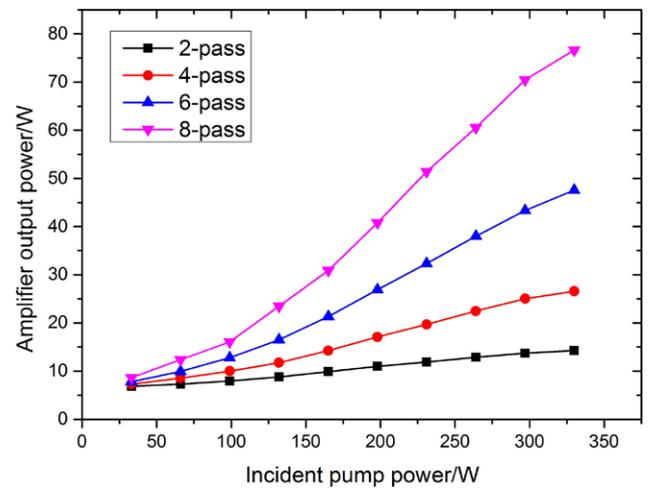
Figure 6. The amplifier output power versus the incident pump power with different even numbers passing through the crystal at 30kHz.
