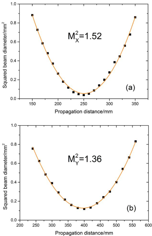
**Figure 7.** The beam quality in (a) the unstable direction and (b) the stable direction.
