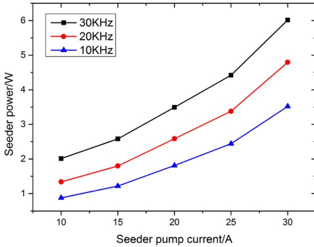
Figure 3. Output power of the seeder laser.
