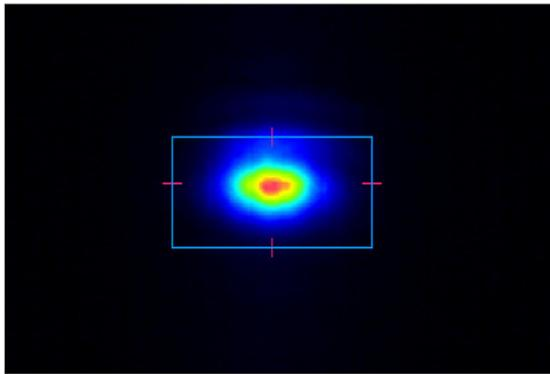
Figure 4. The beam shape of the shaped seeder laser at the amplifier entrance.
