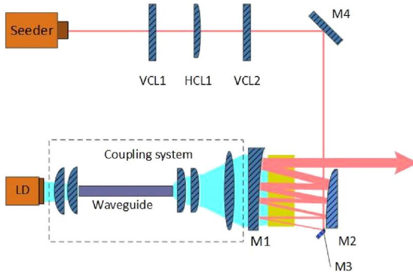
Figure 2. Schematic of the experimental setup.
