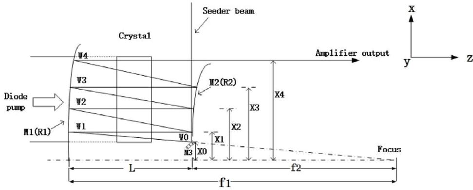
Figure 1. Schematic of the eight-pass slab amplifier geometry.
