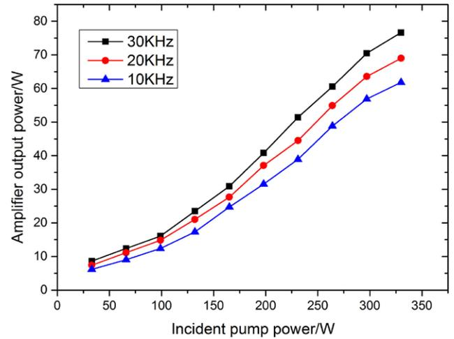
Figure 5. The amplifier output power versus the incident pump power at different frequencies.
