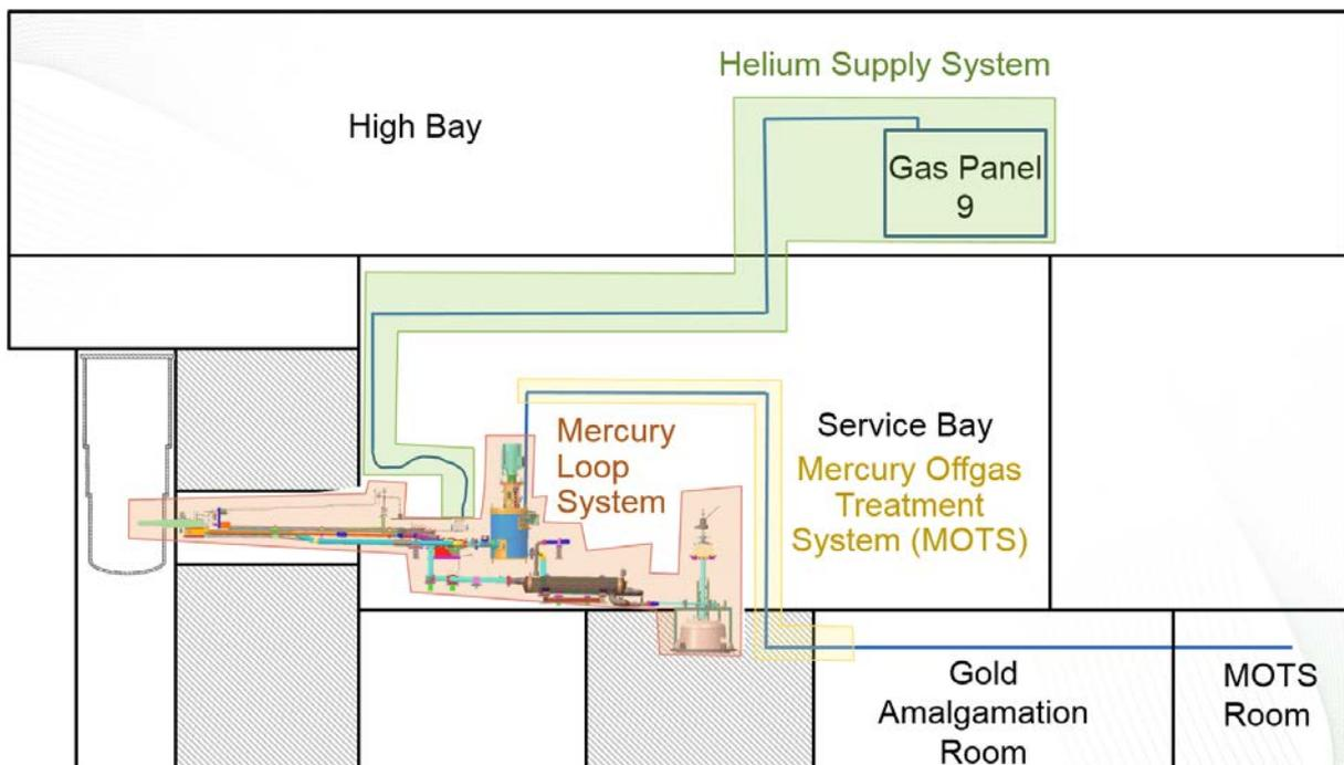
Figure 1 - GI3 Schematic Diagram
