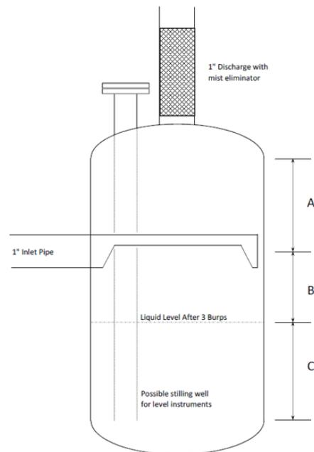
**Figure 5 - Conceptual representation of MOTS GLS**
