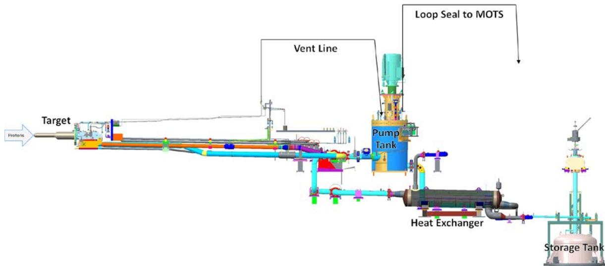
**Figure 3 - Mercury Loop with Major Components**
