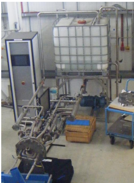
Figure 5 Fig. 5: Current target cooling water flow test rig
