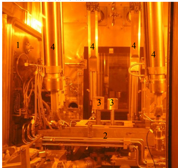
Figure 1 View of RHC from the south manipulator operator room showing 1) void vessel door 2) cantilever beam 3) cryogenic moderators 4) manipulator arms
