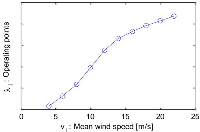
**Figure 3:** Operating points  $\lambda_1$  to  $\lambda_{10}$  corresponding to each mean wind speed in the training data. Online, this table is used for interpolation.
