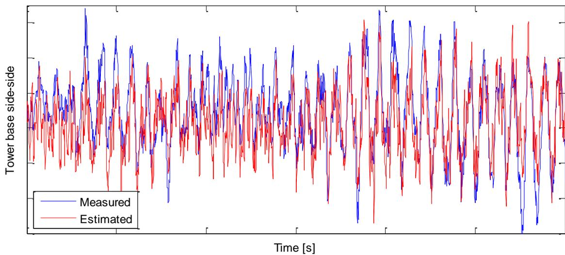
**Figure 6:** Measured and estimated tower base side-side bending moment for the example simulation. The results are zoomed in time to show detail and the time axis labels removed to protect design details because this load component is dominated by rotor speed.
