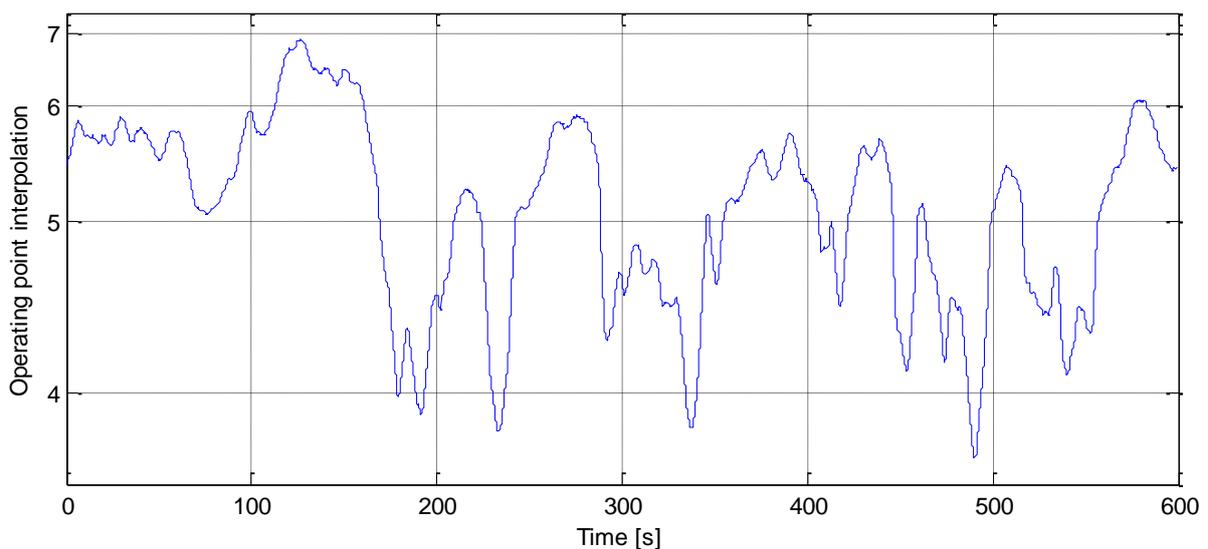
**Figure 4:** Operating point index as it varies over a 600 second simulation at mean wind speed 12 m/s.
