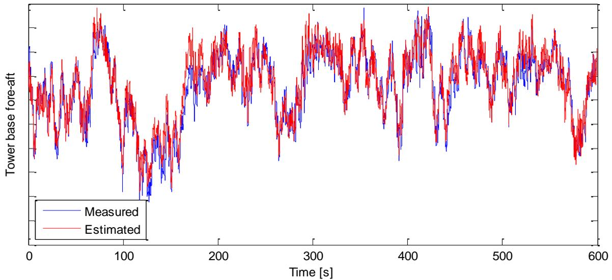
**Figure 5:** Measured and estimated tower base fore-aft bending moment for the example simulation.
