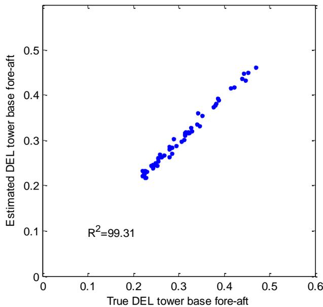
**Figure 10:** Tower fore-aft damage equivalent loads (normalised) from 60 simulations across ten wind speeds from 4 m/s to 22 m/s under normal turbulence conditions, from the load estimator against the true values. Coefficient of determination  $R^2 = 99.31\%$ .
