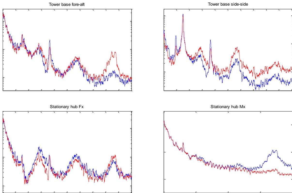
**Figure 9:** Measured (blue) and estimated (red) four load components, for the same simulation as illustrated in Figures 5-8, shown in the frequency domain. Axis numbers have been removed to protect intellectual property.
