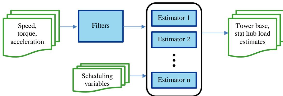
**Figure 1:** Schematic diagram of the load estimator at run time
