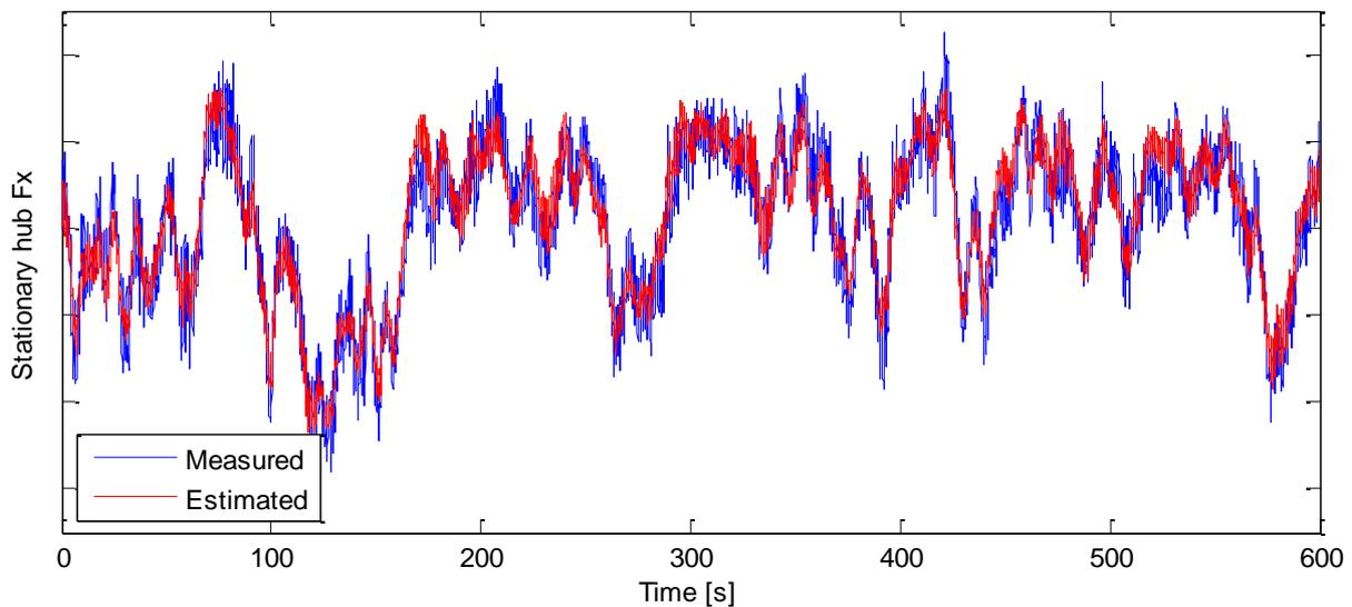
**Figure 7:** Measured and estimated stationary hub Fx (thrust force) for the example simulation.
