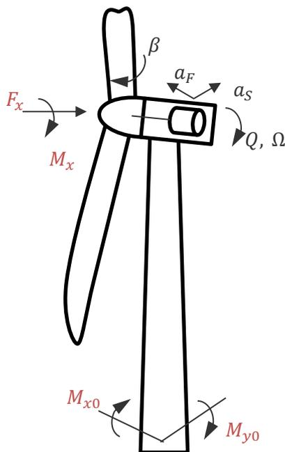
**Figure 2:** An overview of the wind turbine model used in this work. Inputs to the load estimator, known at run time, are  $\beta$  pitch angle,  $a_F$ ,  $a_S$  fore-aft and side-side nacelle acceleration, and  $Q$ ,  $\Omega$  generator torque and speed. Outputs, to be estimated at run time, are  $F_x$ ,  $M_x$  stationary hub thrust and in-plane moment, and  $M_{x0}$ ,  $M_{y0}$  tower base fore-aft and side-side bending moments.
