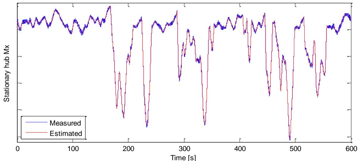
**Figure 8:** Measured and estimated stationary hub Mx (torque) for the example simulation. Note the accurate response of the load estimator during transients such as around 160 seconds.
