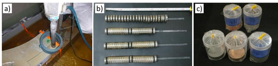
**Figure 2.** Principal processes of sample preparation, a) core samples (diameter: 5 cm, length 3–36 cm) were extracted from the metal components of the cyclotron using a core drill, b) extracted samples were sliced into 1-cm-thick test pieces by a tip saw after the dose rate measurement via a sodium iodide (NaI) scintillation survey meter, and c) each test piece was packed in a plastic container (U8 type) for characterization by  $\gamma$ -ray spectrometry.
