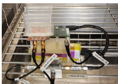
Figure 5. Sensor Prototype inside the climate chamber, with mounted plastic foil and water tank above the electrodes.
