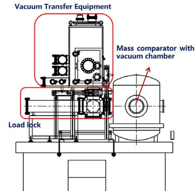
Figure 1. M-one with vacuum transfer equipment
