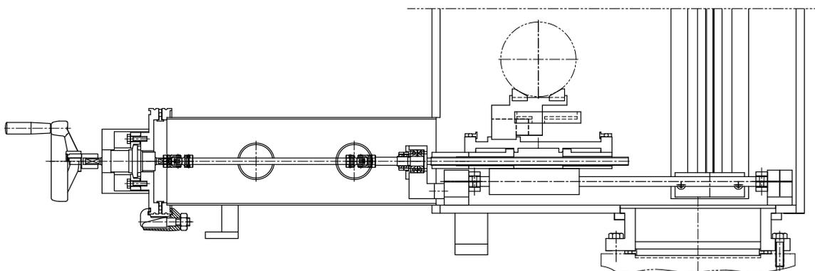
Figure 4. the structure of the horizontal motion manipulator
