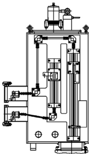
Figure 5. the structure of two vertical motion manipulators
