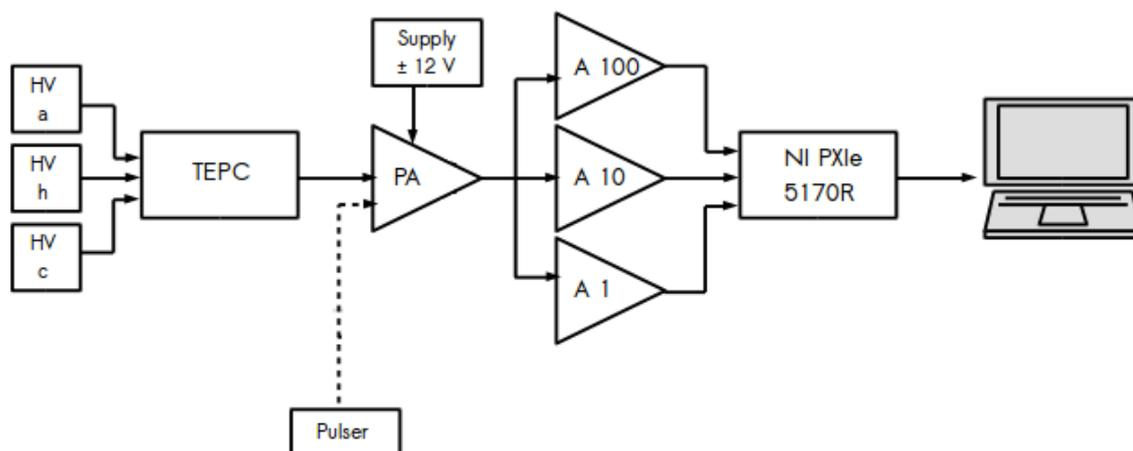
**Figure 1.** Block diagram of the TEPC whole electronic and acquisition chain.
