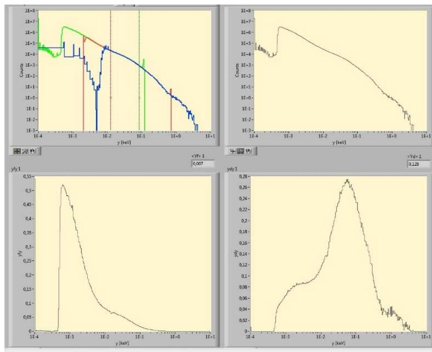
**Figure 2.** Software user interface in which the microdosimetric elaboration is shown. Top-left: spectra from each channel. Top-right: joint and rebinned spectrum. Bottom-left: frequency distribution  $yf(y)$ . Bottom-right: dose distribution  $yd(y)$ . Note that the neutron microdosimetric spectrum shown in this figure is not calibrated against lineal energy.
