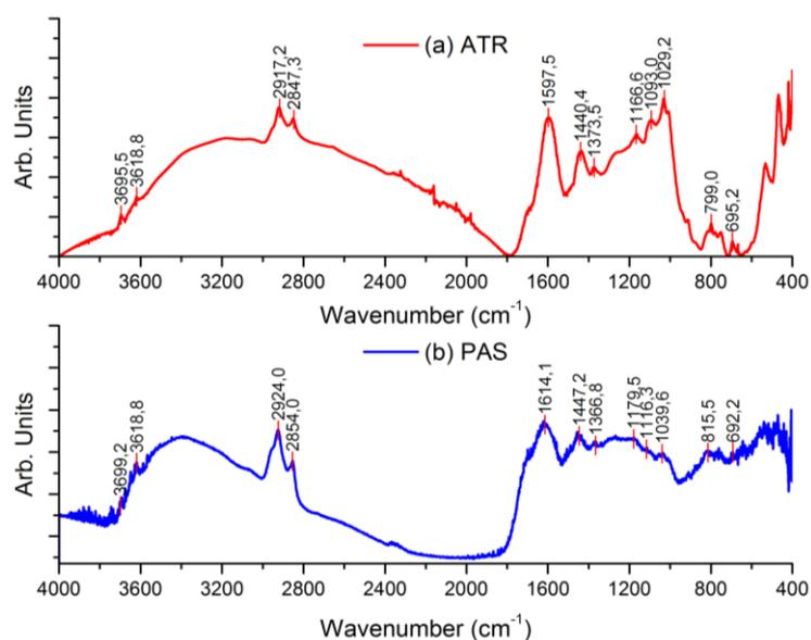
**Figure 2.** Spectra of coal sample from (a) FTIR-ATR and (b) FTIR-PAS measurements at a mirror velocity of 0.16 cm/s, 512 scans and a resolution of  $2\text{cm}^{-1}$ .
