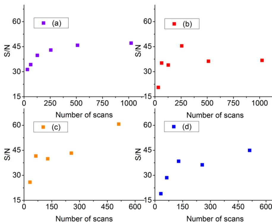
**Figure 1.** Variation of signal-to-noise ratio with spectrometer parameters: mirror velocity ( $v$ ), resolution ( $R$ ), and number of scans. (a)  $v = 0.16\text{ cm/s}$  and  $R = 4\text{cm}^{-1}$ . (b)  $v = 0.32\text{ cm/s}$  and  $R = 4\text{cm}^{-1}$ . (c)  $v = 0.16\text{cm/s}$  and  $R = 2\text{cm}^{-1}$ . (d)  $v = 0.32\text{ cm/s}$  and  $R = 2\text{cm}^{-1}$ .
