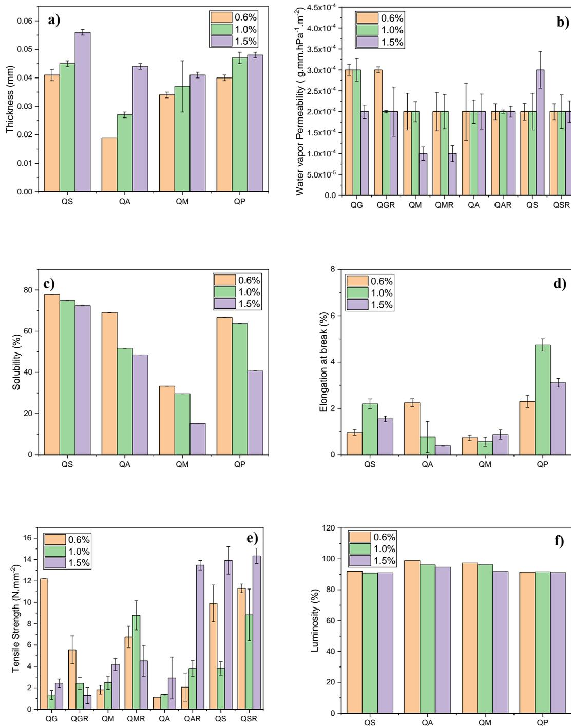
**Figure 2.** Properties (a) thickness, (b) water permeability, (c) solubility, (d) elongation at break, (e) tensile strength and (f) luminosity of prepared chitosan films with different types and concentrations of natural plasticizers and PVA.
