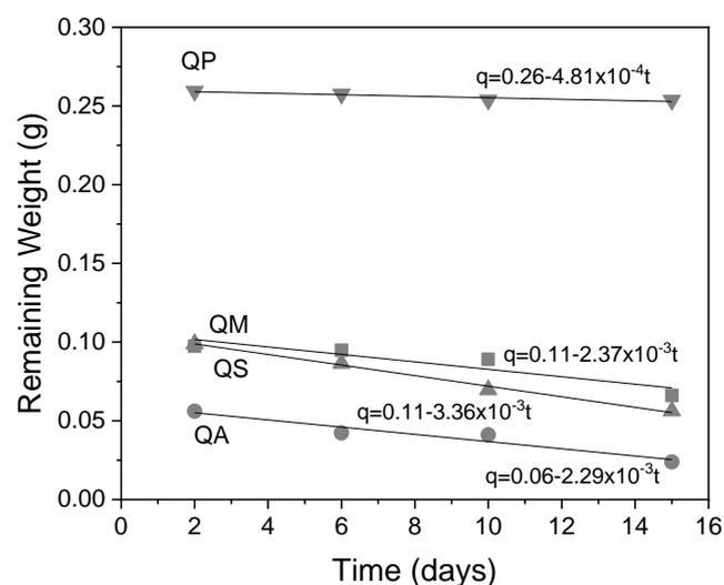
**Figure 3.** Biodegradability in anaerobic conditions of films prepared with natural plasticizers and PVA (1%).
