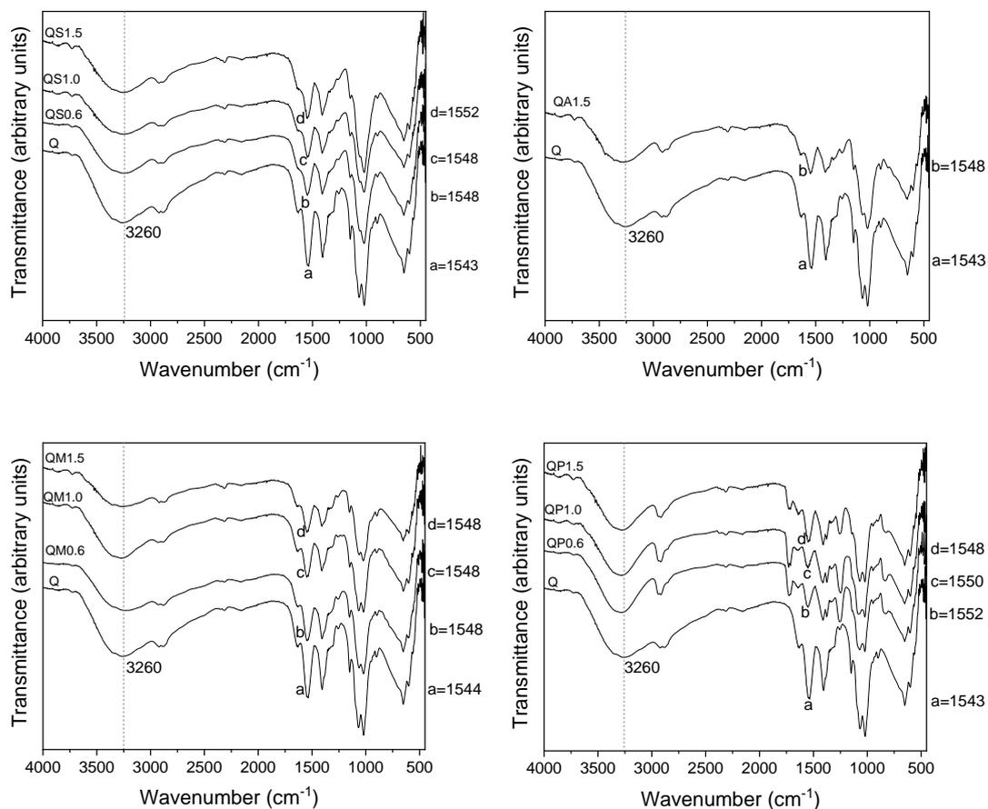
**Figure 1.** FTIR analyses of the films with different types and concentrations of natural plasticizers.
