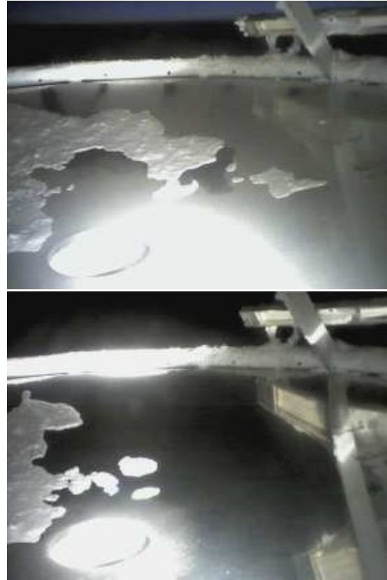
FIG. 4: Images taken by the webcam that monitors the primary mirror. The effect of the heating system is shown: on the left image the mirror appears opaque because it is covered by a layer of frost; after 12 hours of heating, at a set point temperature of few degrees higher than the air temperature, the mirror appears shiny: the frost has been removed.
