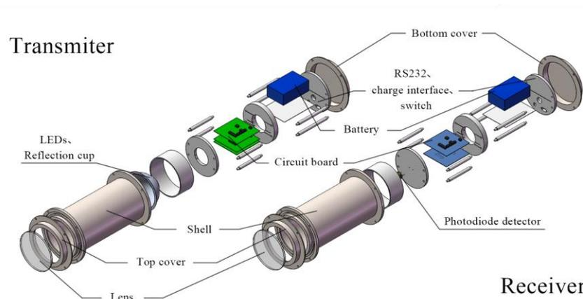
**Figure 2.** Structure of underwater wireless communication system.
