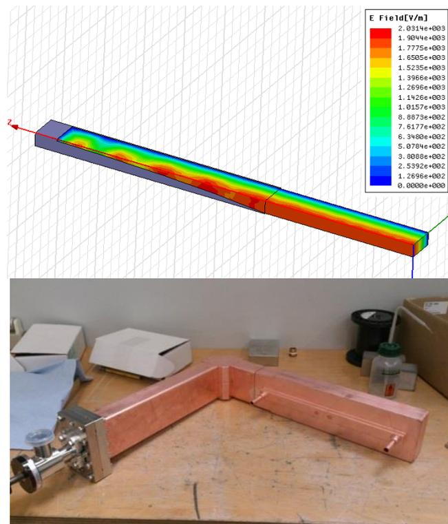
**Figure 5.** The load: distribution of the complex amplitude of electric field in calculation model and photo of load @ E-bend assembly.
