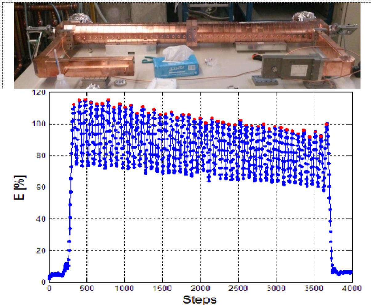
**Figure 7.** Manufactured deflector structure and measured distribution of the amplitude of the deflecting electric field.
