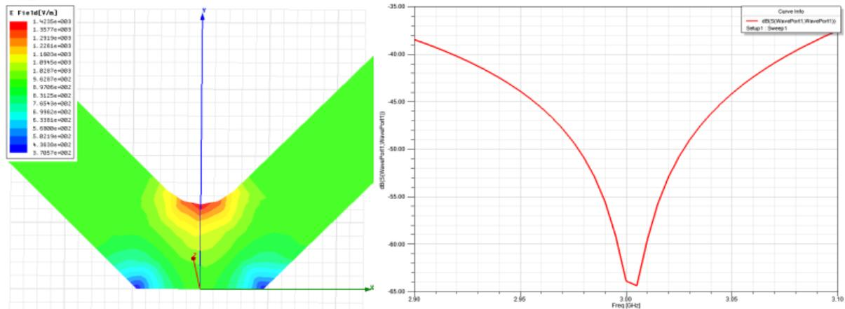
**Figure 4.** E-bend: distribution of the complex amplitude of electric field in calculation model and reflection S11(f).
