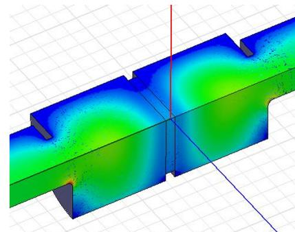
Figure 3. Window: reflection  $S_{11}(f)$  for simulated tuning process (operating curve is brown), distribution of the complex amplitude of the electric field and reflection  $S_{11}(f)$  measured in the built window.  $S_{11} = -45$  dB at operating frequency.
