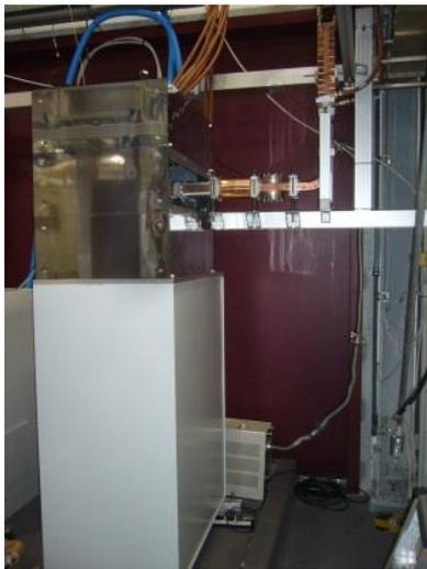
**Figure 1.** Modulator with klystron and local shielding.
