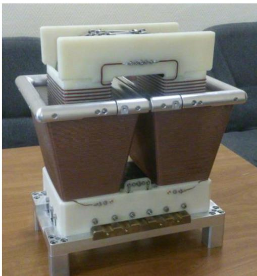
**Figure 5.** Pulse transformer.
