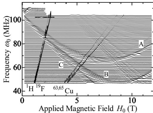
Fig 2. Field-swept spectra of  $^{59}\text{Co}$ -NMR measured with various frequencies  $\omega_0$ . Each spectrum is drawn shifted in proportion to  $\omega_0$ . The small sharp peaks are spurious signal of  $^1\text{H}$ ,  $^{19}\text{F}$  and  $^{63/65}\text{Cu}$  coming from the probe.
