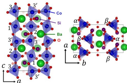
Fig 1. Schematic crystal structure of  $\text{BaCo}_2\text{Si}_2\text{O}_7$ .
