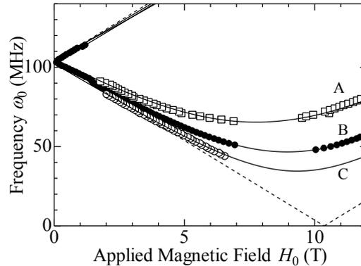
Fig. 3 Signal positions of three Co sites for various NMR frequencies  $\omega_0$ . The dashed line shows the collinear model, and the solid curves, non-collinear one. The fitted parameters are shown in Table 2.
