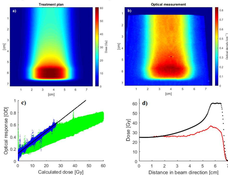
**Figure 4.** Interpolated planned doses (a) and optical measurement (b) for dosimeter C, irradiated with a SOBP entering from above. Correlation plot between plan and measurement is shown in (c), and (d) shows a projection through the central pixels of the plan and the measurement (see figure 3 for further details).
