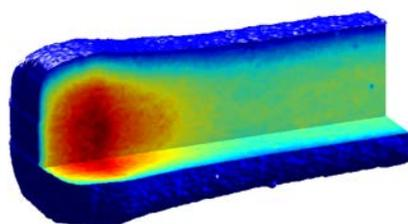
**Figure 2.** 3D view of the optical measurement of dosimeter C. Protons entered from the right. The optical density is scaled from 0.4 cm<sup>-1</sup> (blue) to 0.8 cm<sup>-1</sup> (red).
