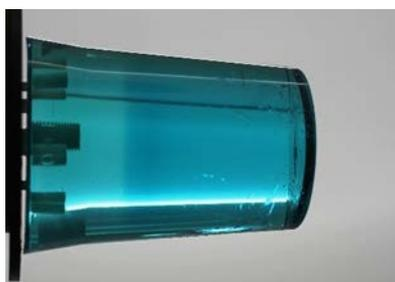
**Figure 1.** A photograph of a dosimeter, irradiated with an SOBP-field, entering from the right.
