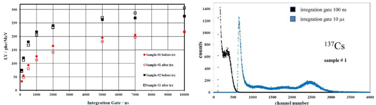
**Figure 1.** (left) Measured light output for two Gd loaded samples as a function of the integration gate of the output of the photomultiplier with bialkali photocathode. The response to a  $^{137}\text{Cs}$  source was measured at room temperature. (right) Response of sample #1 to  $\gamma$ -rays from a  $^{137}\text{Cs}$  source. The signals from the photomultiplier are integrated over a gate width of 100 ns or 10  $\mu$ s, respectively.
