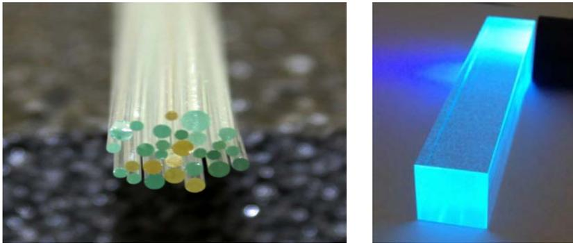
**Figure 3.** (left) Photograph of a bundle of 200 mm long fibers made of DSB:Ce with cross sections of  $\sim 1$ mm. (right) First large volume sample made of DSB:Ce. The rectangular block with a volume of  $23 \times 23 \times 120$  mm<sup>3</sup> has been polished on all surfaces and is illuminated with a UV-lamp.
