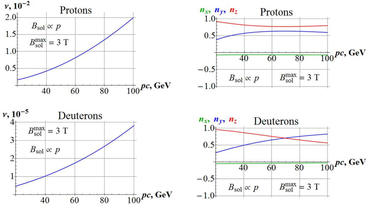
**Figure 4.** Momentum dependence of the spin tune and  $\vec{n}$  – axis components induced by insertion of the detector solenoid for protons (top) and deuterons (bottom). In these calculations, the solenoid field scales proportionally to the beam momentum and reaches 3 T at the maximum beam momentum of 100 GeV/c.
