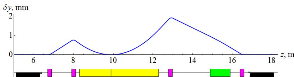
**Figure 3.** Vertical deviation of the ion beam from the axis of the ion straight section. The field of the detector solenoid is 3 T. The beam momentum is 100 GeV/c.
