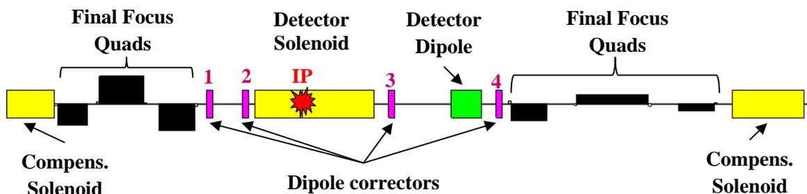
**Figure 2.** Schematic of the detector solenoid placement in the JLEIC ion collider ring.
