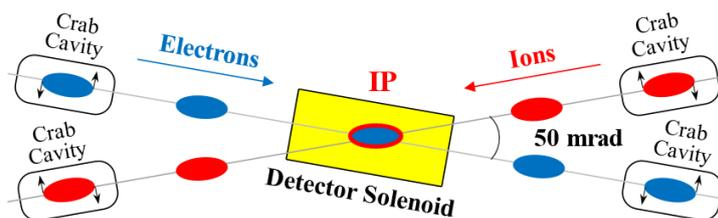
**Figure 1.** Schematic of the detector solenoid placement in the JLEIC ion collider ring.
