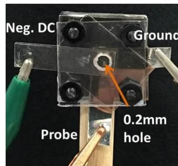
**Figure 2.** A sketch of discharge device. **Figure 3.** A picture of the experimental Hollow-cathode (C), hollow-anode (A), wall probe (P) and mica wall (M).  $200 \mu\text{m}$ .
