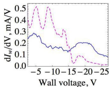
**Figure 5.** First derivative,  $dI_w/dV$ , with respect to wall potential for figure 5. Dashed curve (65- $\mu\text{m}$  device,  $I_d = 6.5$  mA) and solid curve (200- $\mu\text{m}$  device,  $I_d = 8.2$  mA).
