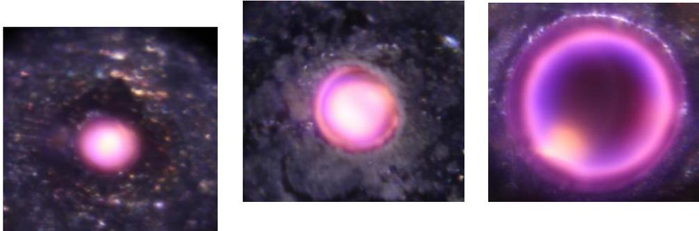
**Figure 1.** Pictures of the devices with the laser produced hole with the diameter of 100  $\mu\text{m}$  (left) and the drill-bit produced hole with the diameter of 200  $\mu\text{m}$  (middle) and 450  $\mu\text{m}$  (right).
