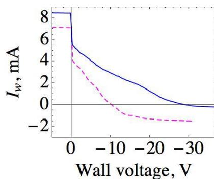
**Figure 4.** Wall current  $I_w$  with respect to wall potential in a Helium dc discharge surrounded by air. Dashed curve (65- $\mu\text{m}$  device,  $I_d = 6.5$  mA) and solid curve (200- $\mu\text{m}$  device,  $I_d = 8.2$  mA).
