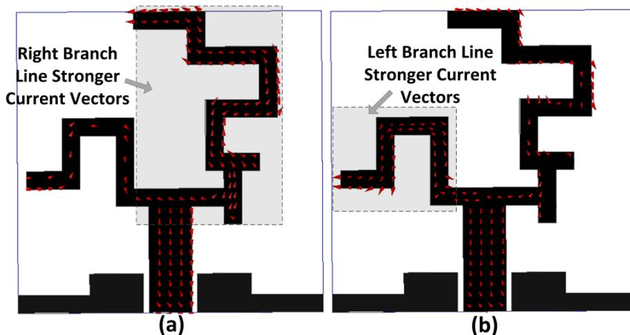
**Figure 3.** Currents on branch lines of the proposed final fractal antenna. (a) Right Branch Line at 1.5GHz (b) Left Branch Line at 5.5GHz.
