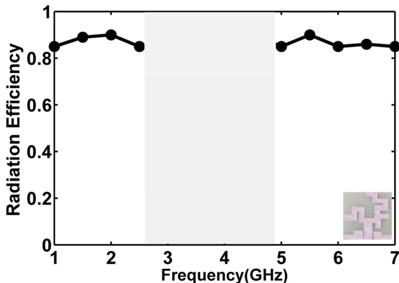
Figure 8. The radiation efficiency of the proposed fractal antenna.
