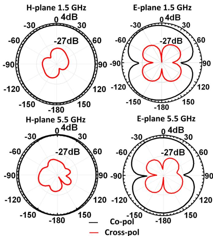
**Figure 7.** The radiation pattern of the proposed fractal antenna.
