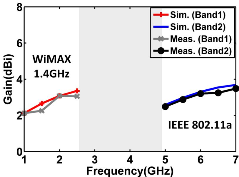
**Figure 6.** Measured and simulated fractal antenna gain for the proposed antenna with dual-band operation.
