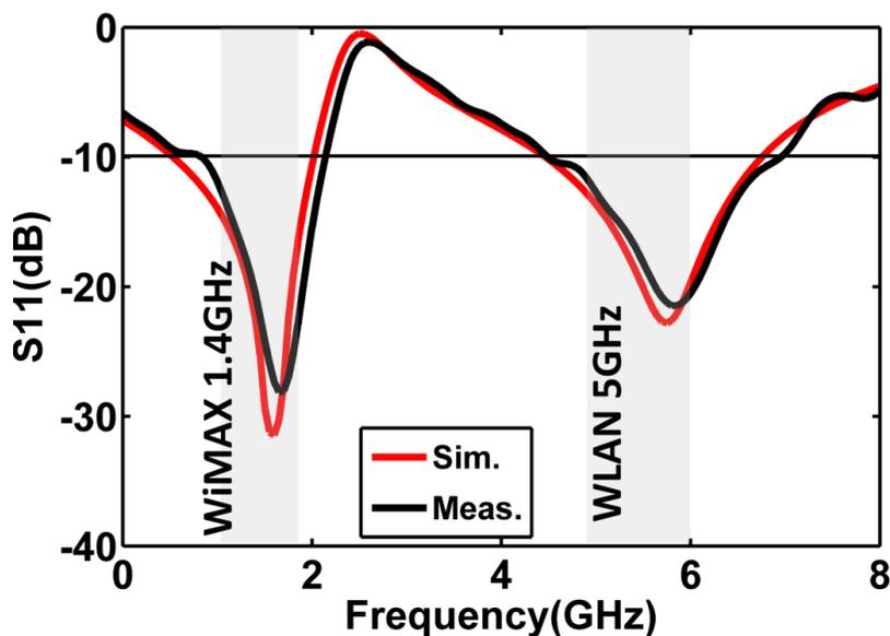
Figure 5. Measured and simulated  $S_{11}$  of the proposed fractal antenna.
