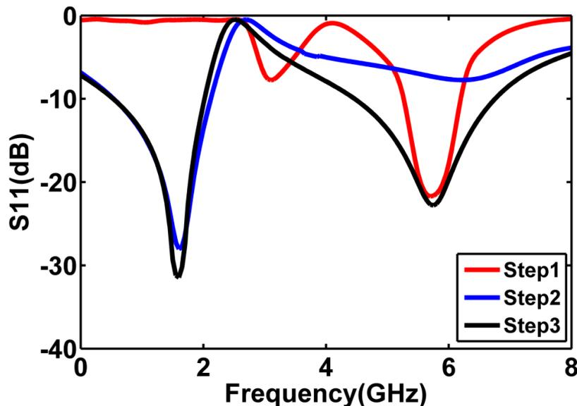
Figure 4. Simulated return loss for final Fractal antenna design steps as shown in figure 2.
