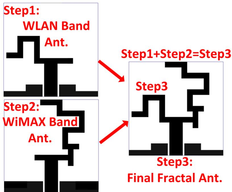
**Figure 2.** Geometry of the proposed final fractal antenna.
