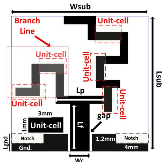
**Figure 1.** Configuration of the proposed dual-band fractal antenna with double branch line made of definite number of unit cells.
