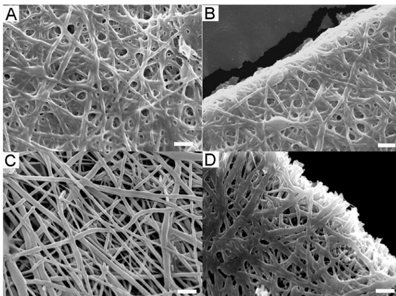
**Figure 5.** Optimized crosslinked samples. SEM images of G18\_3d37B ((A) and (B)) and G18\_1d55B ((C) and (D)). Scale bar = 2  $\mu\text{m}$ .
