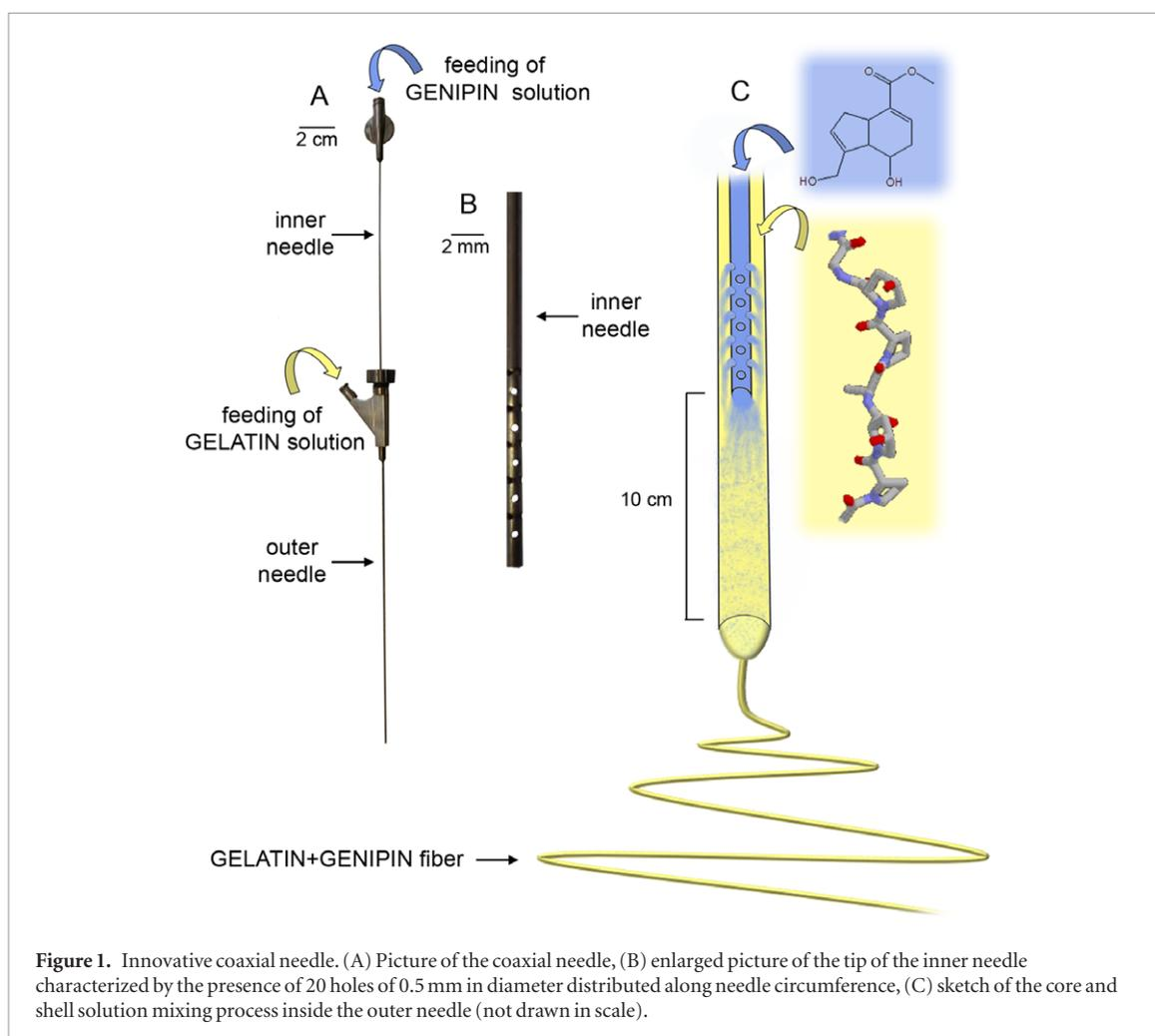
**Figure 1.** Innovative coaxial needle. (A) Picture of the coaxial needle, (B) enlarged picture of the tip of the inner needle characterized by the presence of 20 holes of 0.5 mm in diameter distributed along needle circumference, (C) sketch of the core and shell solution mixing process inside the outer needle (not drawn in scale).
