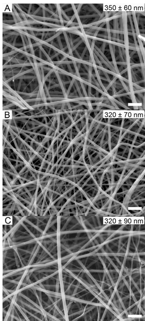
**Figure 2.** SEM micrographs of as-spun electrospun mats. (A) G9, (B) G18 and (C) GEL. Fiber mean diameter and standard deviation are reported for each sample. Scale bar =  $2 \mu\text{m}$ .
