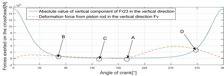
**Figure 7.** Comparison of  $F_{r23} \cos \varphi$  and  $F_v$  with  $\theta$  being the x-coordinate
