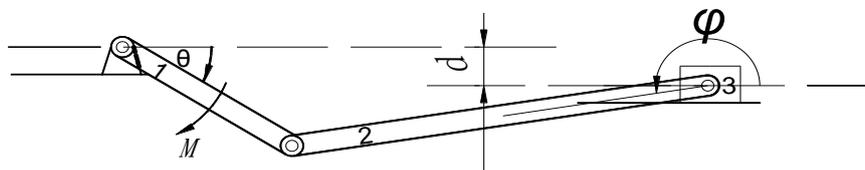
**Figure 1.** schematic diagram of the crank-slider mechanism
