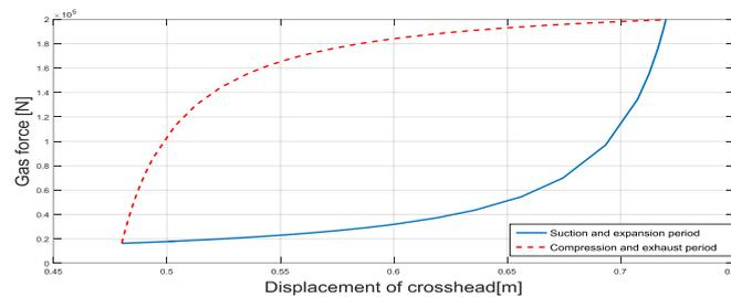
**Figure 5.** Gas force acted on the piston rod ( $F_h$ )
