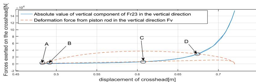
**Figure 6.** Comparison of  $F_{r23} \cos\varphi$  and  $F_v$  with  $x_3$  being the x-coordinate
