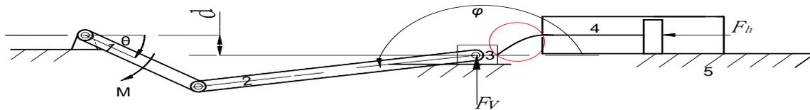
**Figure 3.** Schematic of the mechanism considering the influence of piston rod and the gas force
