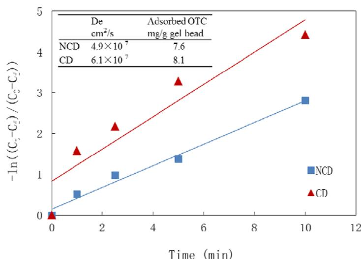
**Figure 1.** Cumulative mass transfer capacity of OTC into gel beads (NCD and CD represent gel beads without and with CD)
