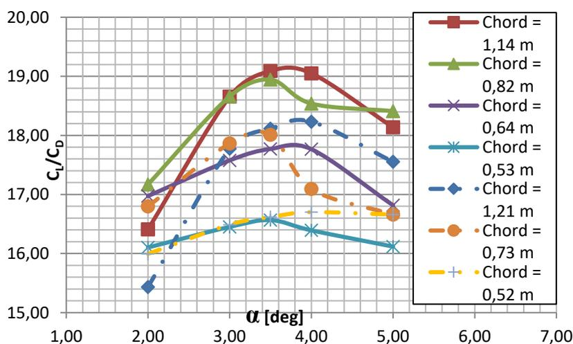
**Figure 5.** Lift-to-drag ratio as function of angle of attack for foils with 5-m span and different chord's lengths.
