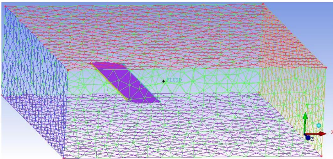
**Figure 3.** Position of the foil in the computational domain.
