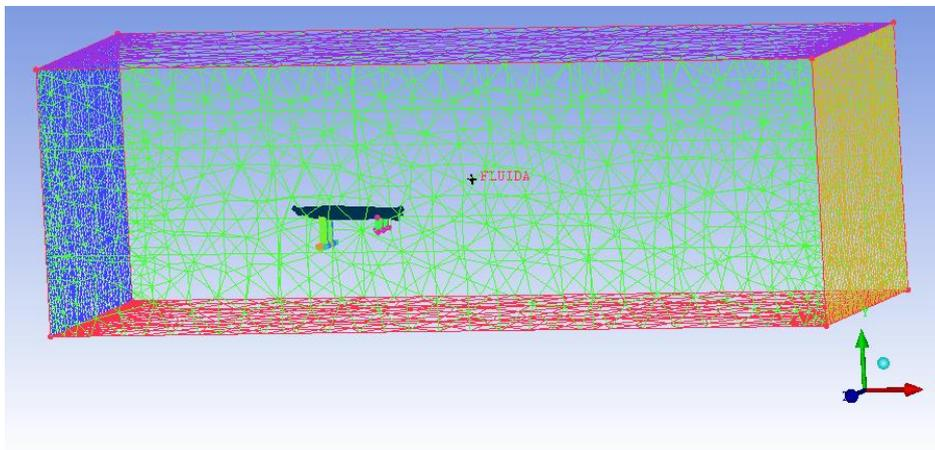
**Figure 7.** Position of the hydrofoil-raft model in the computational domain.
