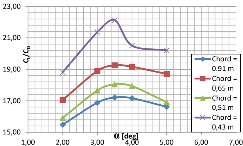
**Figure 4.** Lift-to-drag ratio as function of angle of attack for foils with 4-m span and different chord's lengths.
