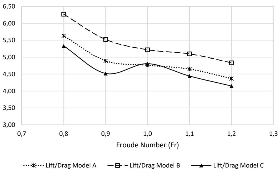
**Figure 9.** Lift-to-drag ratio of the hydrofoil craft for model A, B and C.
