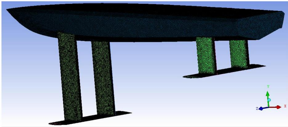
**Figure 6.** Mesh of the hydrofoil craft for model B.
