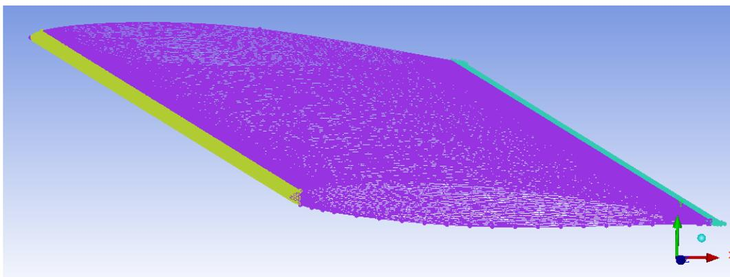
**Figure 2.** Mesh of NACA 64(1)212 foil used for the hydrofoil craft.
