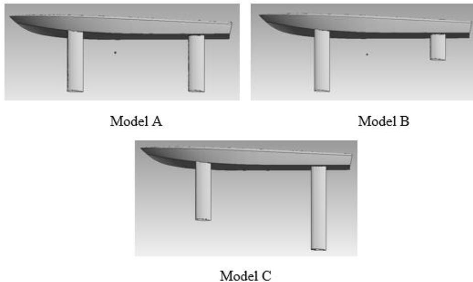
**Figure 1.** Three alternatives for the stern-foil submerged elevation with constant front-foil elevation.
