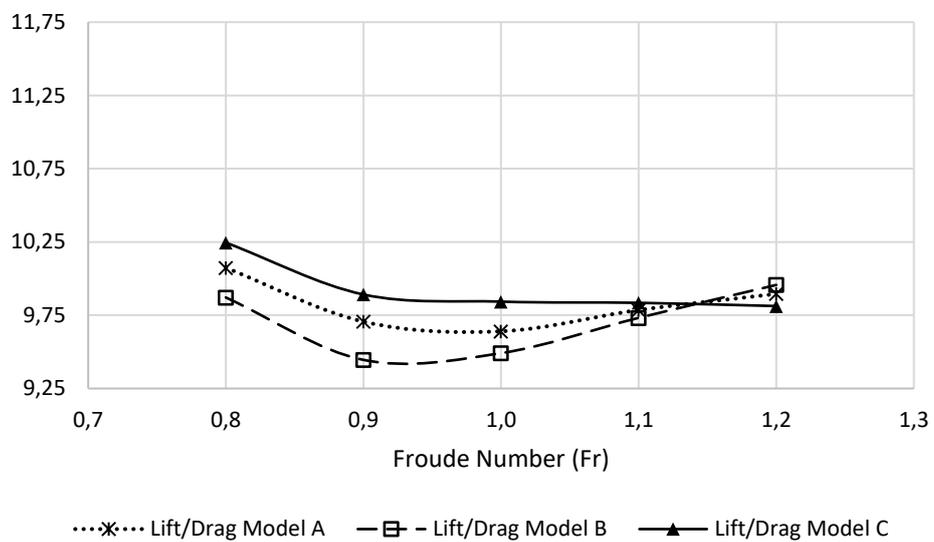
**Figure 8.** Lift-to-drag ratio of the stern foil for model A, B and C.
