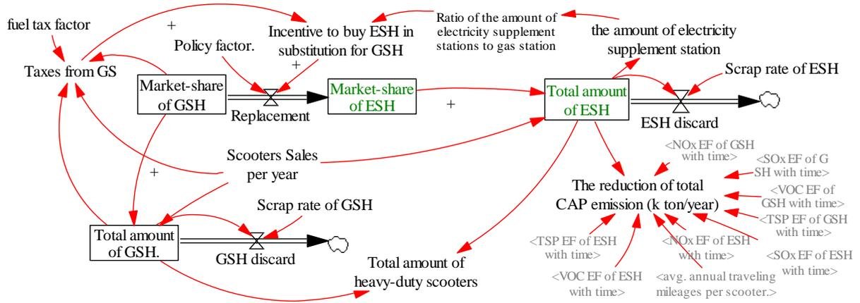
**Figure 1.** Simplified causal loop and stock-and-flow diagrams for GS and ESH stock.
