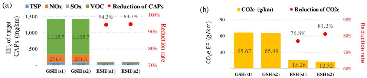
Figure 2. Comparison of EF<sub>k</sub> for GSH and ESH (in s1 and s2).
