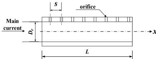
Figure 1. Simplified model of drip irrigation pipe.
