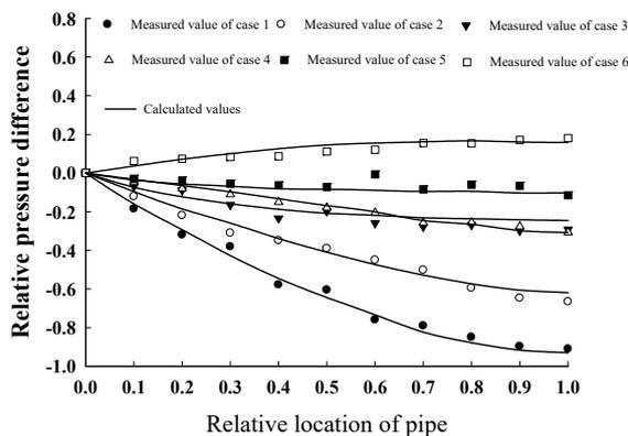
Figure 6. Comparison of longitudinal static pressure distribution between measured and calculated values.
