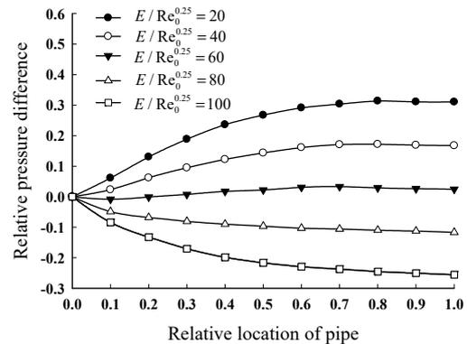
Figure 7. Relationship between  $E / Re_0^{0.25}$  and longitudinal static pressure distribution.
