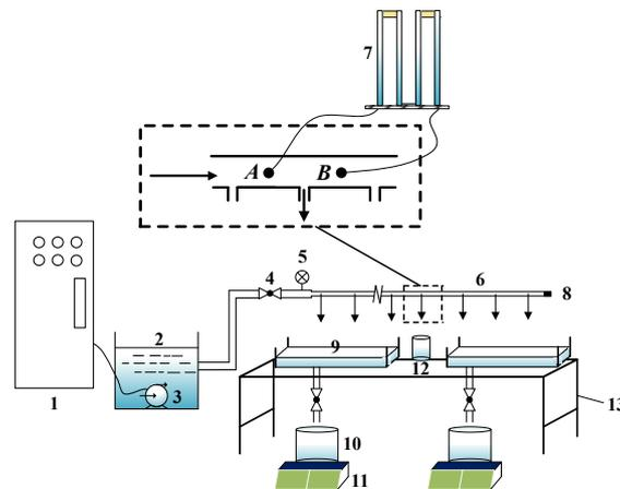
1. Variable frequency cabinet 2. Reservoir 3. Centrifugal pump 4. Globe valve 5. Pressure gauge 6. Drip pipe 7. Manometer 8. Plug
