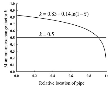
Figure 4. Relationship between  $m$  and  $N$ . Figure 5. Axial variation of momentum exchange factor.
