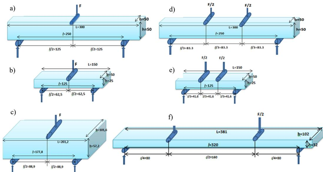
**Figure 1.** Test arrangement for a) EN 12372 (50\*50\*300mm) b) EN 12372 (25\*50\*150mm) c) ASTM C 99 d) EN 13161 (50\*50\*300mm) e) EN 13161 (25\*50\*150mm) f) ASTM 880-98
