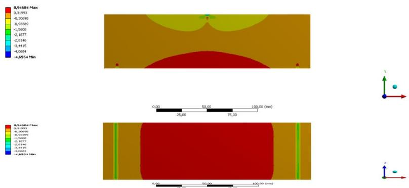
Figure 5. ASTM C99 a) frontal surface b) lower surface normal stress distribution
