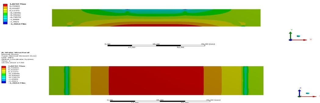
Figure 7. EN 13161\_25\*50\*150 mm a) frontal surface b) lower surface normal stress distribution
