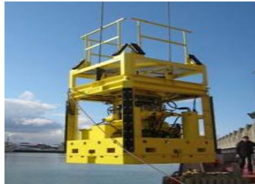
Figure6 Submarine static penetration testing device MANTA-200
