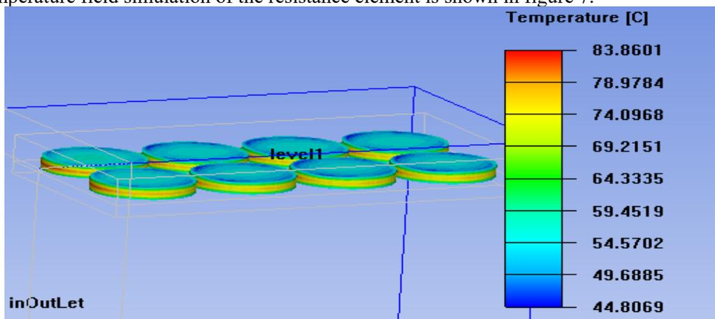
Figure 7. Temperature distribution graph of the resistance elements
