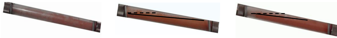
Displacement velocity 2.5mL/min, oil recovery 10.3% Displacement velocity 0.5mL/min, oil recovery 7.5% Displacement velocity 0.05mL/min, oil recovery 8.4% Figure 3. oil-gas interfacial at different displacement velocity
