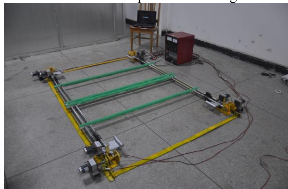
Figure 1: Prototype of electronic controlled bamboo dance mechanism
