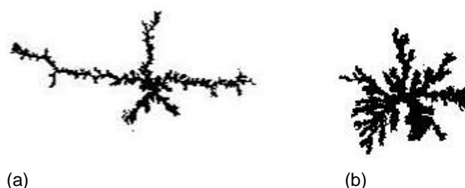
Figure 4. Copper electrodeposits (applied voltage 6 V, \text{CuSO}_4 0.2 M, time duration 20 minutes): (a) without magnet, (b) in strong magnetic field [18]
