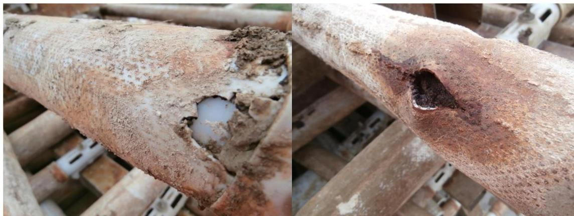
**Figure 4.** Corrosive effect of  $\text{FeCl}_3$  about aeration system
