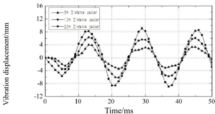
**Figure 4.** Vibration displacement of perforating string at different positions.
