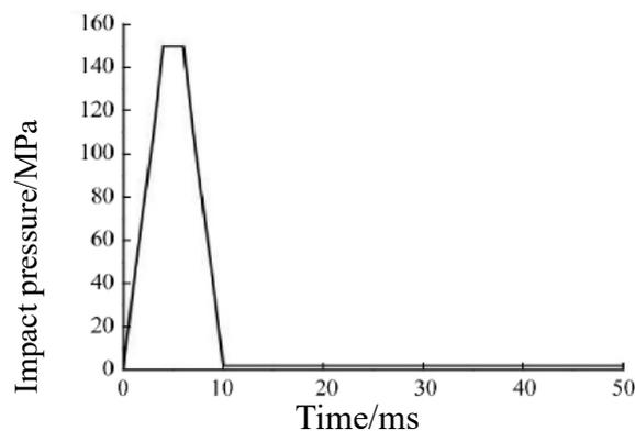
**Figure 3.** Axial shock load by perforating.
