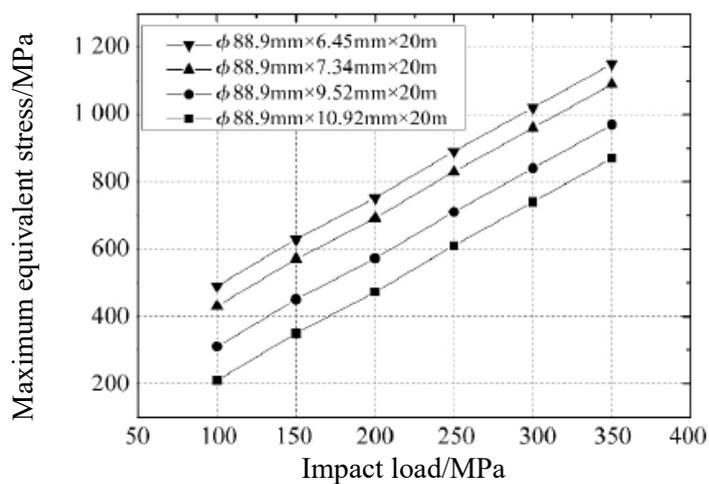
Figure 10. Maximum equivalent stress of columns with perforations of different wall thicknesses under different amplitude perforation impact loads.
