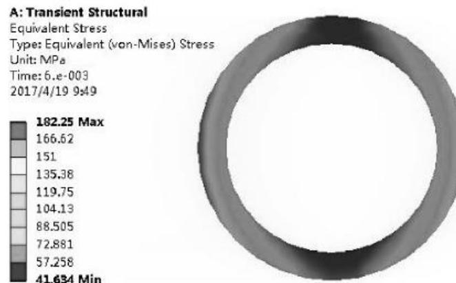
Figure 7. Equivalent stress distribution near packer at 6 ms.
