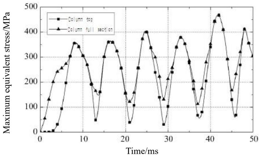
Figure 9. The maximum equivalent stress of string versus time.
