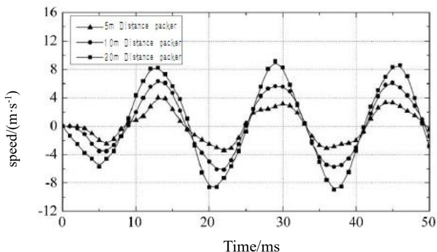
**Figure 5.** Vibration velocities of perforating string at different points.
