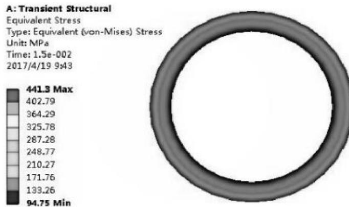
Figure 8. Equivalent stress distribution near packer at 15 ms.
