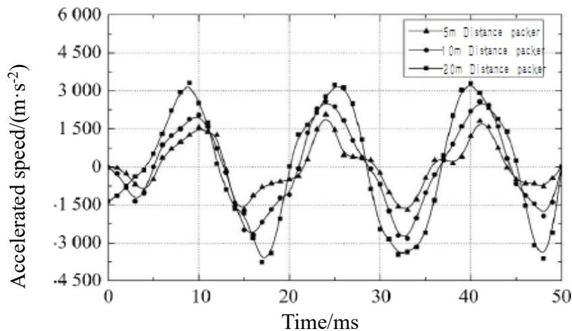
Figure 6. Vibration velocities of perforating string at different points.
