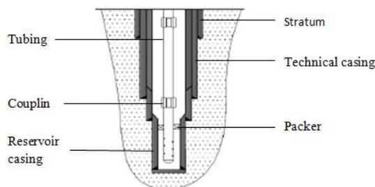
**Figure 1.** Schematic diagram of tubing conveyed perforating string.
