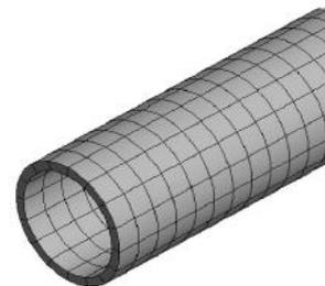
**Figure 2.** Local diagram of finite element model of the perforated strings.
