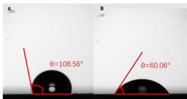
**Figure 2.** the contact angle measurement of  $\text{Si}_3\text{N}_4$  after and before hydrophobic treatment
