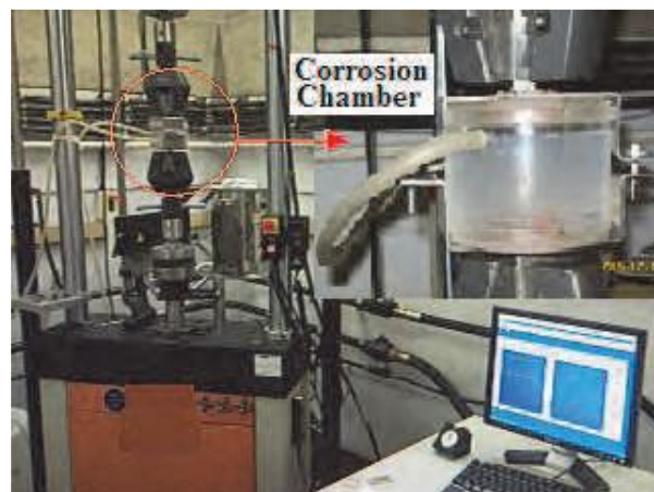
Figure 9. Corrosion fatigue testing in a NaCl solution
