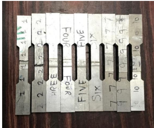
Figure 16. Welded Specimen for Tensile Test
