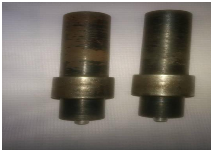
Figure 4. H13-Friction Stir Tooling Circular and Threaded profile
