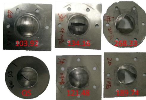
**Figure 6.** Specimens after QS and HSR bulge tests (unit of impact velocity: m/s).
