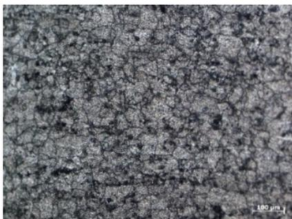
**Figure 1.** Microstructure of 5A06-O.
