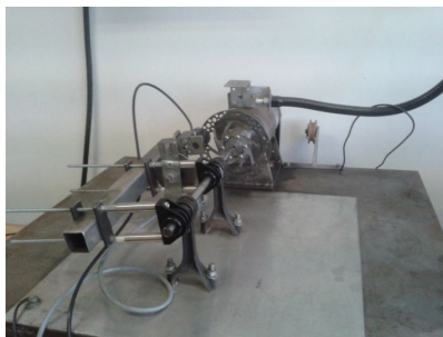
Figure 1. The test stand with brake disc rotor
