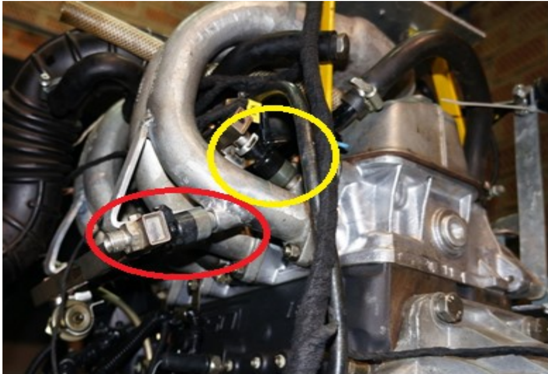
Figure 1. A view of the intake manifold mounted on engine with gasoline injectors (marked in yellow) and additional ethanol injectors (marked in red)
