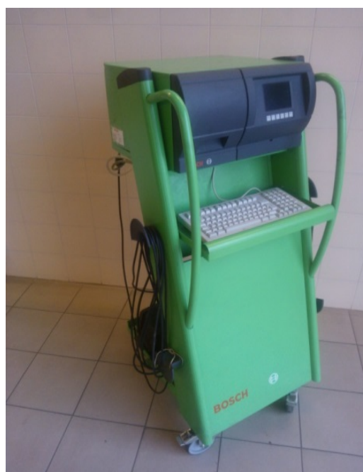
Figure 7. A view of Bosch BEA 350 emissions analyser
