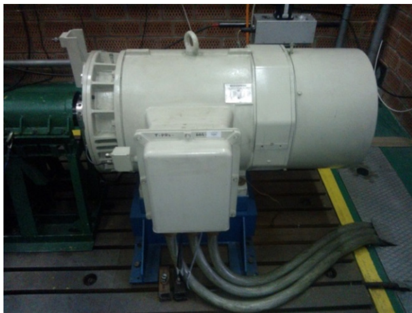
Figure 3. A view of SCHENCK DYNAS 2 220 AC-machine brake
