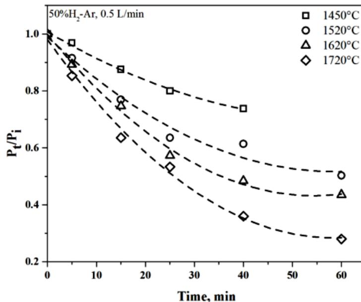
Figure 2. Effect of time and temperature on dephosphorization
