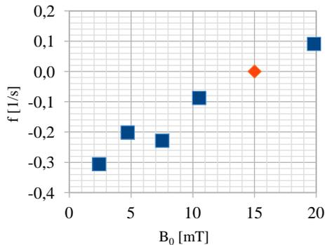
Fig. 3: Circling frequencies  $f$  of the jet for different magnetic flux densities  $B_0$  of the RMF.
