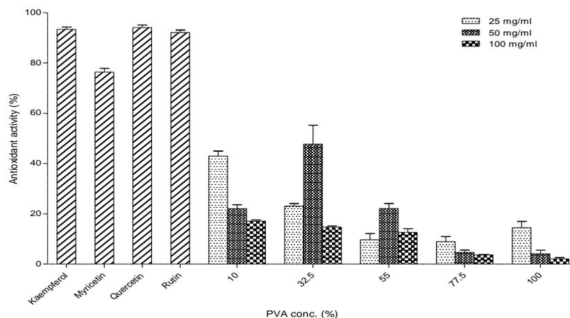
**Fig. 2** Antioxidant activity of *S. palustris* flour-95% HD PVA blends film at different concentrations of the PVA and different dilution rate of the film. Values are the means  $\pm$  SEM (n = 4).
