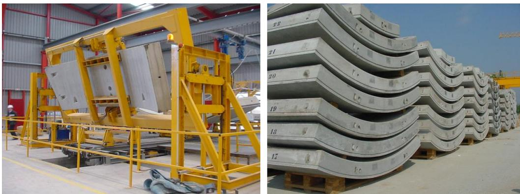
**Figure 4.** Some of the transient load situations in which the segments are subjected to bending moments: (a) demoulding and (b) stacking at the yard
