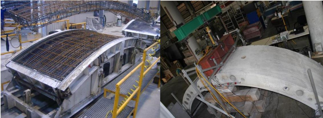
**Figure 3.** Precast concrete segments: (a) Traditional reinforcement (Metro L9 of Barcelona) and (b) FRC full – scale bending test carried out at the UPC of Barcelona
