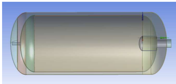
Figure 1. Three dimensional finite element model of gas cylinder.
