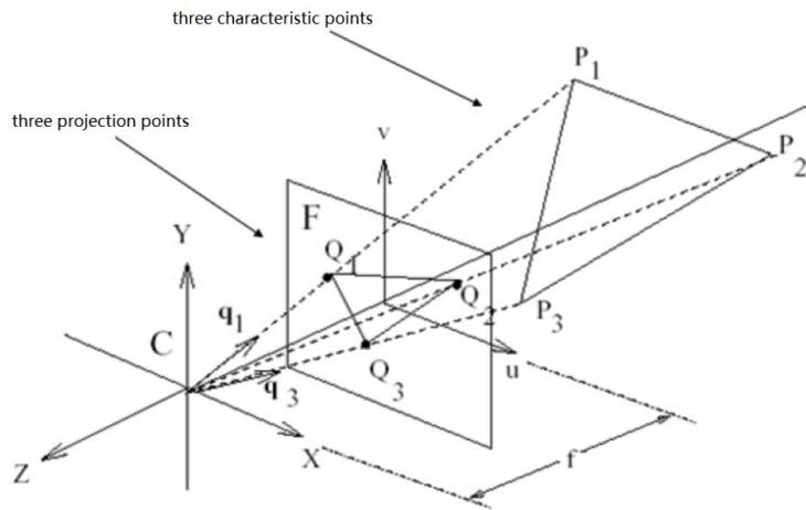
**Figure.1** projection model of head tracking system
