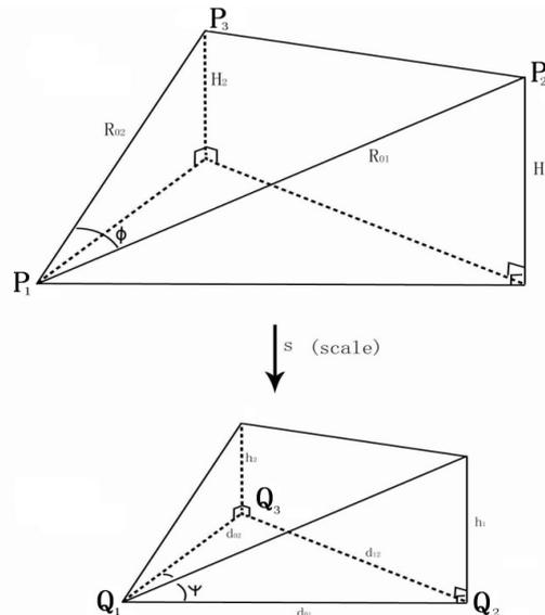
**Figure 2.** Schematic diagram of the relationship between characteristic points and projection points
