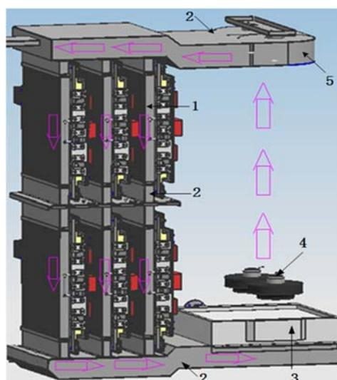
1-radiator; 2-wind tunnel; 3-air-water heat exchanger;
